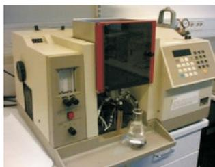
Figura 72. Espectrofotómetro de Absorción Atómica. Tomado de: [http://en.wikipedia.org/wiki/File:Atomic\\_absorption\\_spectroscopy.jpg](http://en.wikipedia.org/wiki/File:Atomic_absorption_spectroscopy.jpg)
