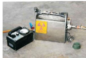
Figura 54. Fuente de rayos gamma. Tomado de: [http://www.ettesting.com/db\\_RTXDevice1.jpg](http://www.ettesting.com/db_RTXDevice1.jpg)
